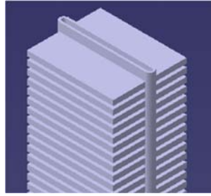
Figure 2.3 Isometric view of Design 1 with rectangular shape of fin with increased thickness.
