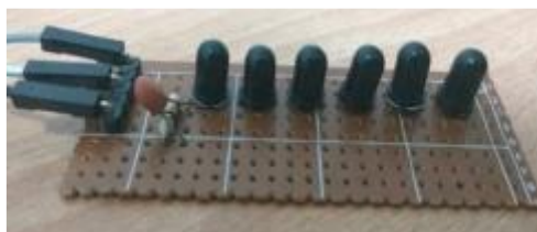
Figure 2. IR LED Receiver Circuit
